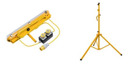
Quick and easy to deploy, the Weatherguard LED 20W Light with Emergency 3hour Battery are mounted on a folding tripod stand offering ultimate flexibility on site. Comes complete with 2x110v 16amp power outlets and 5m of cable.
